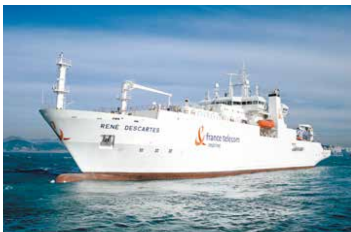
CABLE LAYING SHIP
